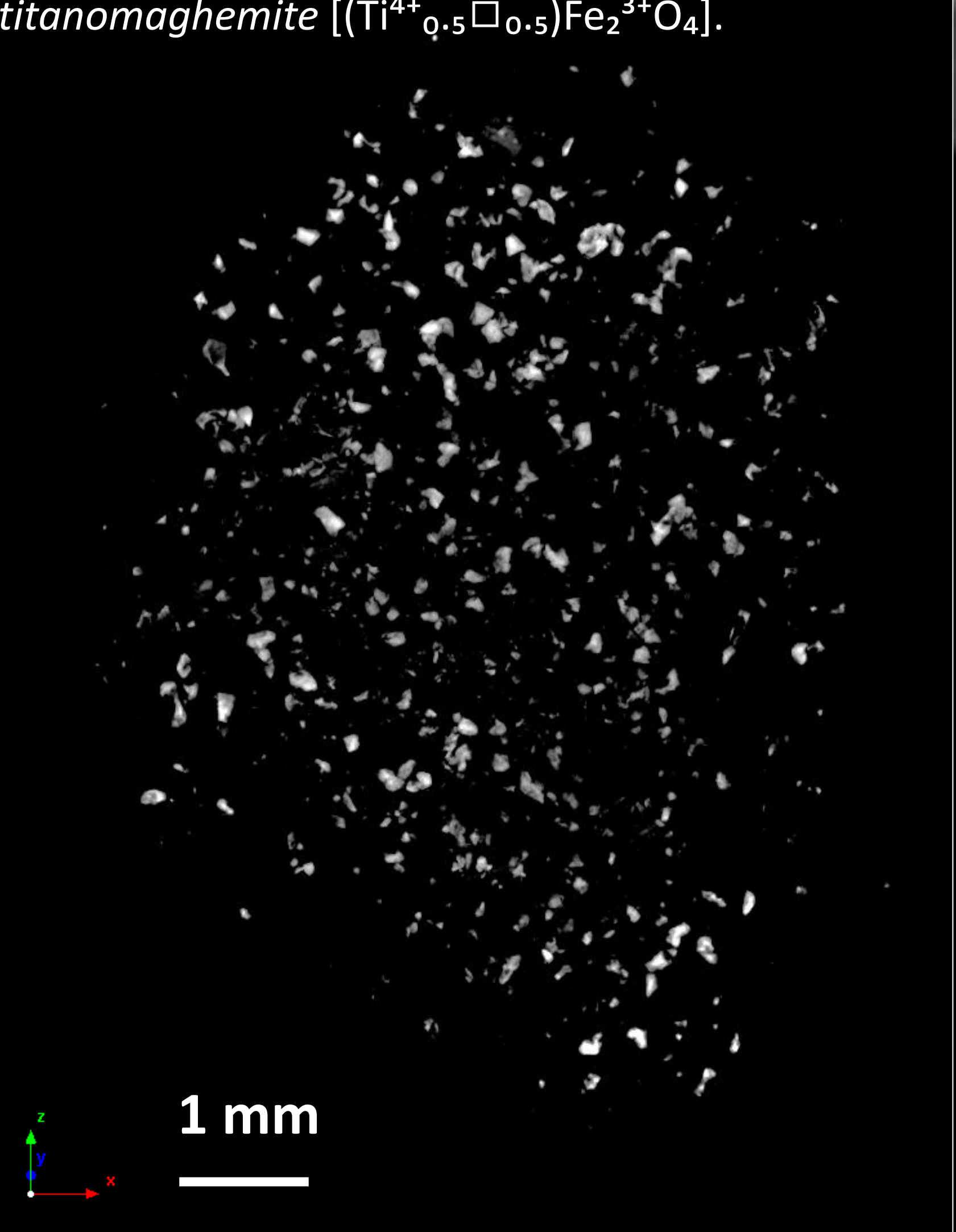
Brightest (i.e., densest) phases may correspond to titanomaghemite [(\text{Ti}^{4+}_{0.5}\square_{0.5})\text{Fe}_2^{3+}\text{O}_4] .
