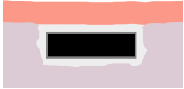
Fig. 2: Illustration of desired pellet configuration in situ. Black is the metal implant, in the experiment case just a dummy metal made from the same material as the real implant as in the in-vivo case. Dark grey is the bioglass coating on the surface of the implant, light grey is the hand-pressed outer pellet made from bioglass powder. The surrounding grey should depict the skull bone and the fleshy pink should depict the skin of the patient.
